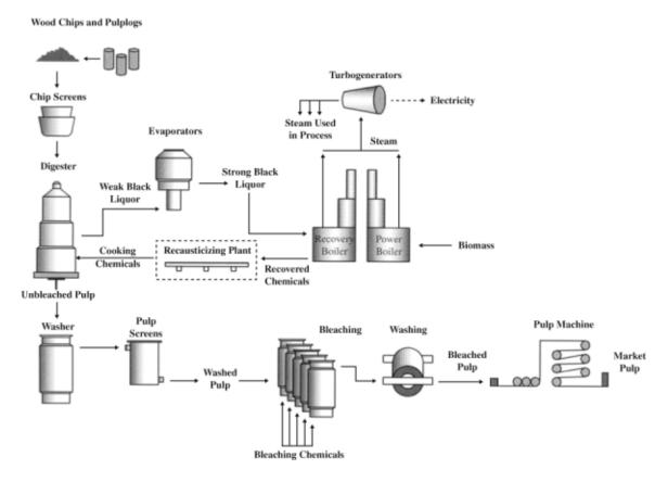
In order to transform wood chips into kraft pulp, wood chips undergo a multi-step process involving the following principal stages: chip screening, digesting, pulp washing, screening, bleaching and drying.
